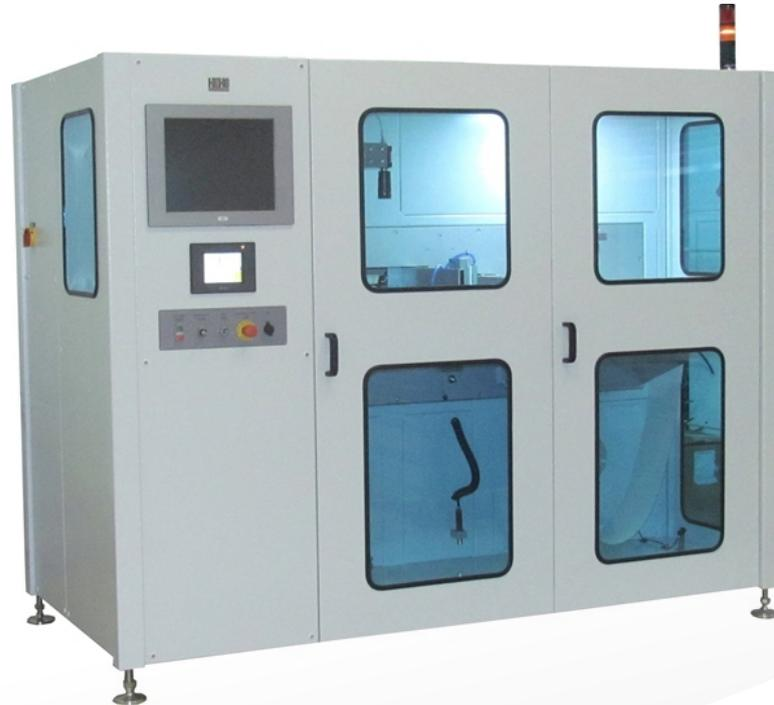
Automatically blanks single sheets from a roll of green tape
