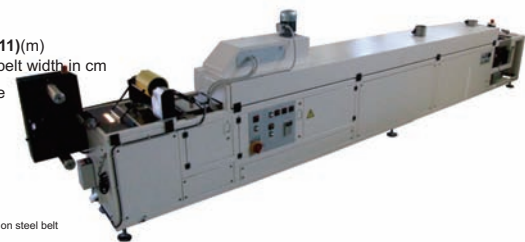
Tape casting on steel belt
