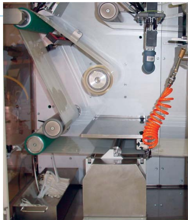
Laser thickness measuring installed on CAM-M1 casting machine
