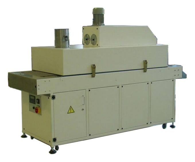
Tunnel type sheet dryer is designed to dry individual ceramic sheets after printing. High air flow ensure high drying efficiency. Sheets are transported by stainless steel chain trough a heating tunnel. Two 6x6 (8x8) inch sheets can be placed on to the drying chain next to each other to increase the drying time. Adjustable internal and fresh airflow circulation.
