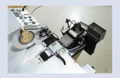
Capacity: up to 40.000 pcs / hour for 8 mm tape dimensions
